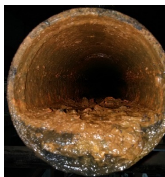
Oxygen Corrosion in Dry Pipe Main
