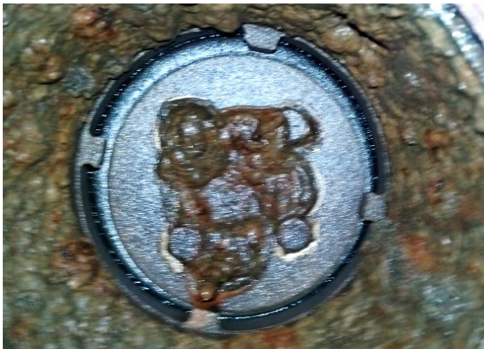
Condensate Corrosion on Underside of Clapper
