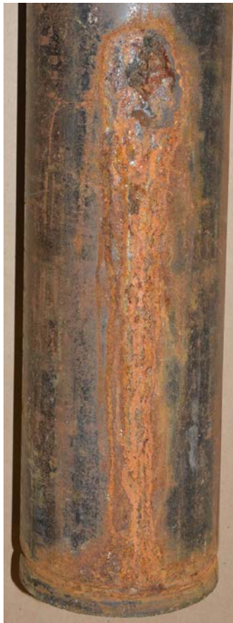
Oxygen Corrosion of Riser Piping (external view at pinhole leak)
