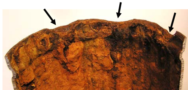
Oxygen Depleted Zone at Rolled Groove of Riser Piping
