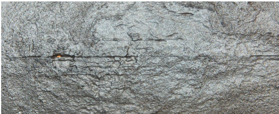
Oxygen Corrosion of Riser Piping with pinhole leak at weld seam (external view)
