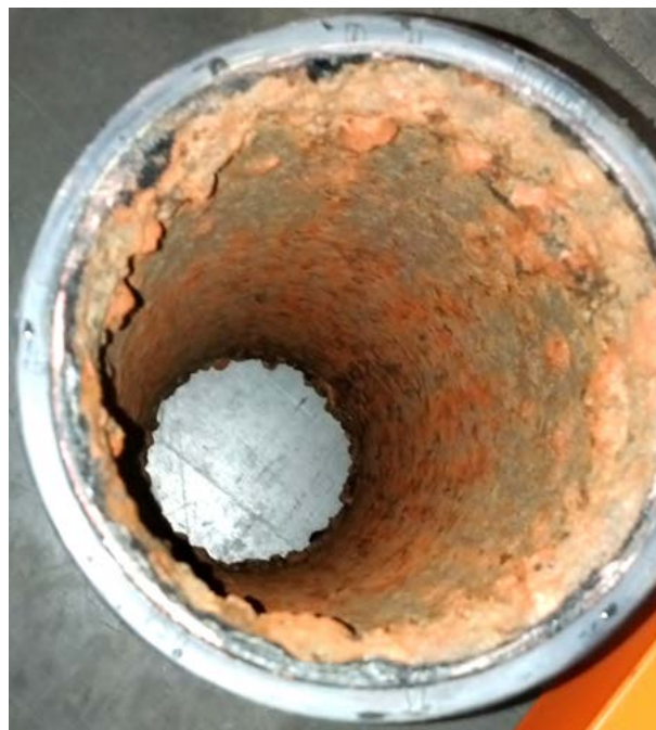
Oxygen Corrosion of Riser Piping
