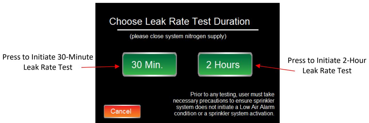
**NOTE:** **Cancel** button stops the Leak Rate Test and returns to Individual Sprinkler System Detail Screen.
