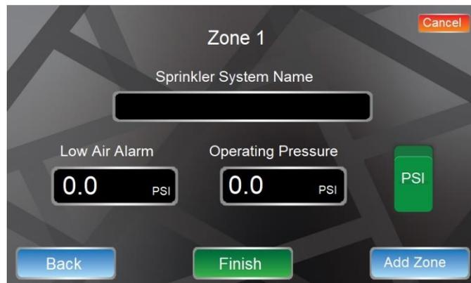
7. Enter the installation location information into the HMI Screen (*Recommended but not required*).
