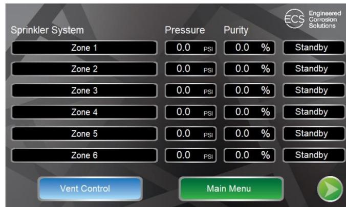
3. Press the **Vent Control** button to initiate fourteen (14) day nitrogen inerting process for any or all sprinkler zones.
