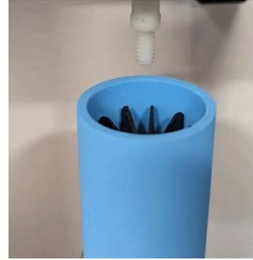
6. Replace with new 5-Micron Coalescing Filter, reinstall black filter plate. Black plastic filter plate should be finger/hand tight.
