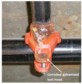
threads and moves by capillary action into the seal between the threads and the fittings. Corrosion will occur at this surface each time the surface is wetted by condensate water and will continue for as long as the surface remains moist. Over time corrosion by-product (hematite) will build up at the point of corrosive attack to hold moisture on the pipe surface which acts to accelerate the rate of metal loss.
