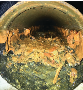
Dry Pipe Systems Trap Water
