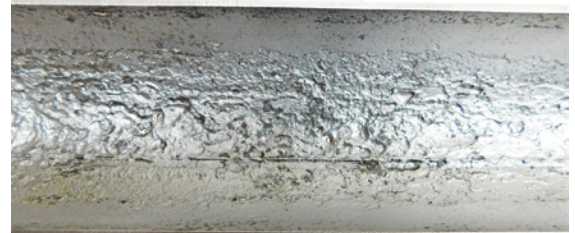
after media blasting
